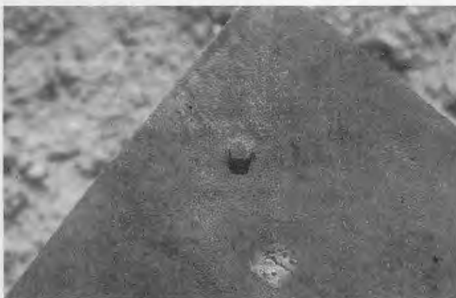
With its penetrator, 5.56mm M855 does serious damage to rifle-grade steel targets. Here a core of the plate was literally pushed part way out the back of the plate.
